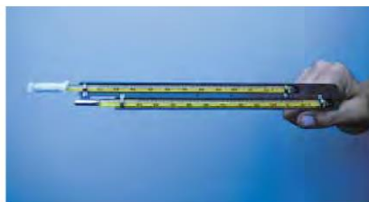
FIGURE 4.9 The sling psychrometer.
